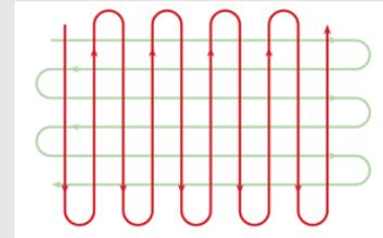
Complete evaporation occurs after approx. 1-2 min. If drops form on the component or the applied matting remains "wet" for longer, increase the spraying distance or increase the spraying speed. The ideal ambient temperature is 21°C/69.8°F.
