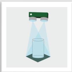
After complete drying of AESUB green, the object can be scanned as usual.
