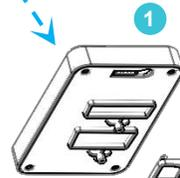
★ 1. Fix the touch screen assembly on the screen holder.
