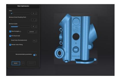
Use recommended parameters: To get FreeScan UE help you optimize a specific model, enable the function. To customize parameters, disable the function.
