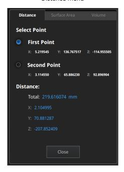
Total is the 3D distance, X, Y and Z are the projection of the segment to the respective planes.
