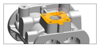
The modern Interactive Solid Modeling feature allows modification of solid geometries, both native and imported, and helps users overcome the parametric logic made of profiles and constraints and the object creation sequence, to get the expected modification result directly. Thanks to its solid modeling and surfacing functionalities, ThinkDesign Engineering ensures innovative part modeling functionalities in a flexible and easy-to-use design environment.
